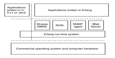
Figure 1: The OTP system architecture
