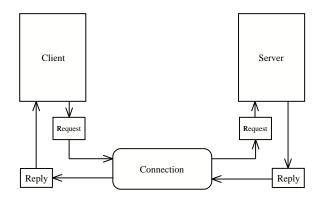
Figure 5: The structure of the client-server design pattern
