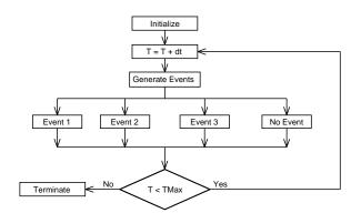
Figure 10: The structure of the Time-Driven Design Pattern
