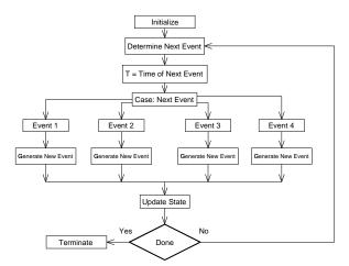
Figure 11: The structure of the Event-Driven Design Pattern
