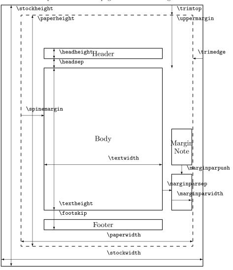
Figure 5: Right-hand page major layout parameters for the memoir class
