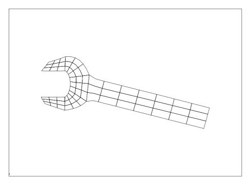
Enlarge the wrench's mouth by zooming for defining the two nodes which will get the load representing the torque (to simplify matters it is assumed, that the screw gets only selectively a couple of forces as torque at the corners and that the screw itself and not the wrench revolves):
