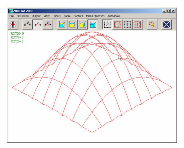
See how the boundaries raise between the corner nodes? Guess we must swallow the bitter pill and support <u>all</u> the nodes laying on boundaries (copy file *B18\_2.TXT* to Z88I2.TXT). This results in:
