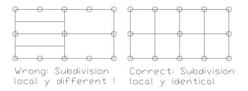
Because the local axises x, y and z are defined by the location of the local nodes 1, 4 and 5, it is possible to generate almost arbitrary numberings for nodes and elements of the FE structure by corresponding construction of the coincidence list in the mesh generator input file Z88NI.TXT.
