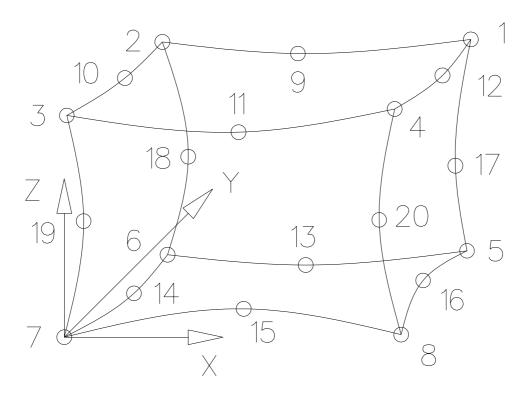
The nodal numbering of the element No.10 must be done carefully and must exactly match the sketch below. Pay attention to the location of the axis system ! The possible error message " Jacobi determinant zero or negative " is a hint for incorrect node numbering.
