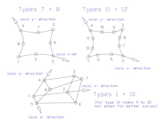
**Example:** Subdivide an Isoparametric Serendipity Plane Stress Element with 12 nodes (Element No.11) into finite elements of type Isoparametric Serendipity Plane Stress Element with 8 nodes (Element No.7). Subdivide in local x direction three times equidistantly and subdivide 5 times increasing geometrically in local y direction. The super element is supposed to have the number 31. Thus :
