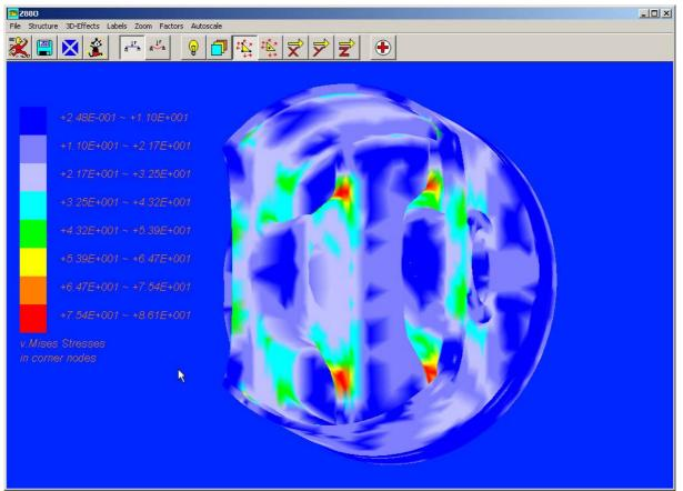
Windows: plot of the von Mises stresses in the corner nodes of the BMW piston.
