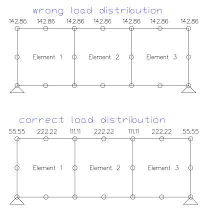
A FE structure consists of three plane stress elements No.7 with the load of 1,000 N distributed on the upper edge in Y direction. Above incorrect, below correct load sharing:
