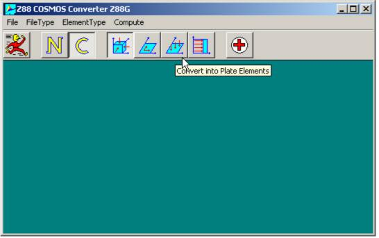
(Before running the conversation choose the right type of elements; works similar for the UNIX version of Z88G in console mode)
