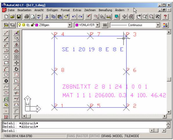
(Windows: AutoCAD LT 97, drawing the rectangular plate)
