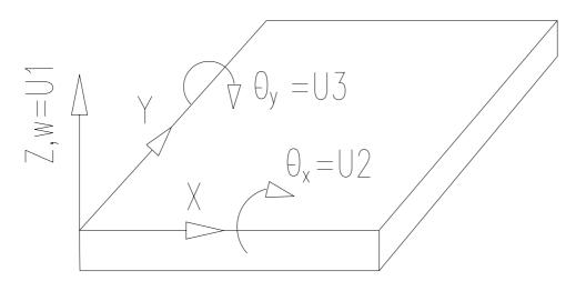
If you want to support the boundary in front, i.e. running in X direction, with cutting edges, then you must fix the degree of freedom 1 (the Z direction) and the degree of freedom 3 (the rotation around the Y axis).
