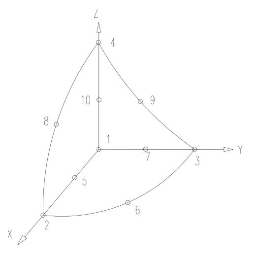
The nodal numbering of the element No.16 must be done carefully and must exactly match the sketch below. Pay attention to the location of the axis system ! The possible error message " Jacobi determinant zero or negative " is a hint for incorrect node numbering.
