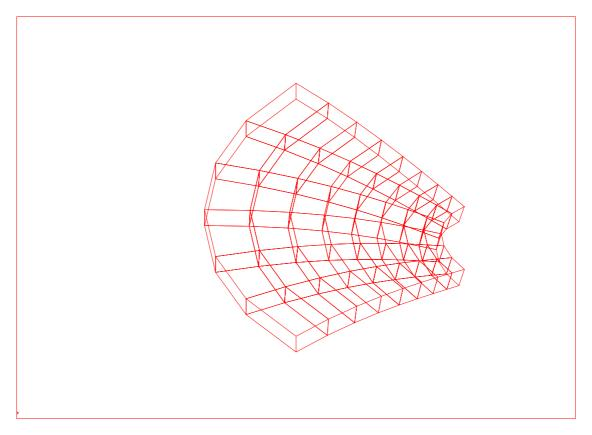
**Hint:** The super structure is very easy to design with e.g. AutoCAD. Draw the edges using arcs. The nodal points can easily be produced by the function > Draw > Point > Divide. When outlining the elements using the LINE function be sure to position the view in space exactly to match all nodes of a super element properly. This is a common source for a later malfunction of the CAD converter Z88X !
