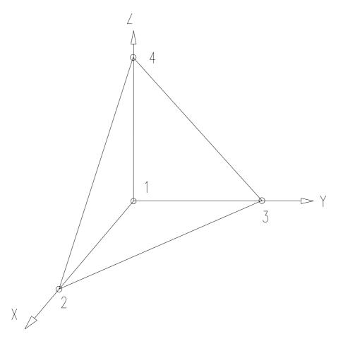
Tetrahedron No.17 cannot be generated by the net generator Z88N. A DXF data exchange with Z88X is not implemented because tetrahedrons due to their strange geometry are very difficult to arrange in space. This element's main purpose is the use with automeshers from third-party suppliers. **Caution:** Sometimes the automeshers of CAD systems produce very bad element and nodal numbering resulting in an useless large amount of memory needs of Z88F. In this case, renumber especially the nodes.
